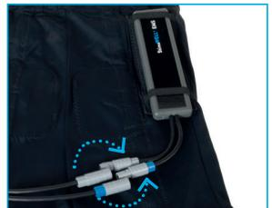
Connect distributor and connection cable. Turn only slightly until the fastener engages (Caution! Pay attention to the colours: blue to blue and grey to grey).
