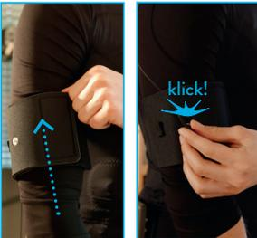
Slip over upper arm electrodes and connect to short cable.
